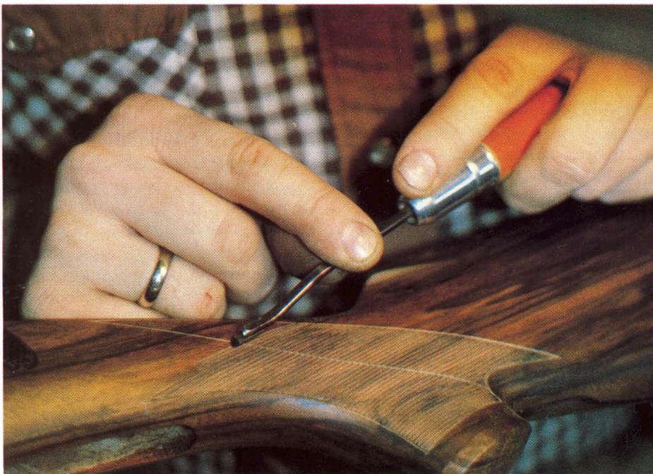
Once a walnut log is cut into slabs, the gunstock begins to take shape. A template is used to trace gunstock outlines on slabs (left). Band sawyers then convert the slabs to gunstock blanks, which are rough shaped by fixed routers as the blanks slowly rotate in carving machines (right). After butt plates and fittings are attached, stocks are smoothed with hand-held sanders (below right) and checkering is carved into the wood (below center). Gunstocks are sold according to grade (below left); common grade, fiddle-back figure, and the highly valuable feather figure illustrate the variable range, and expense, of gunstock options available to gun buyers. (Photo at left by John Strickler; all other photos by Mike Blair)
