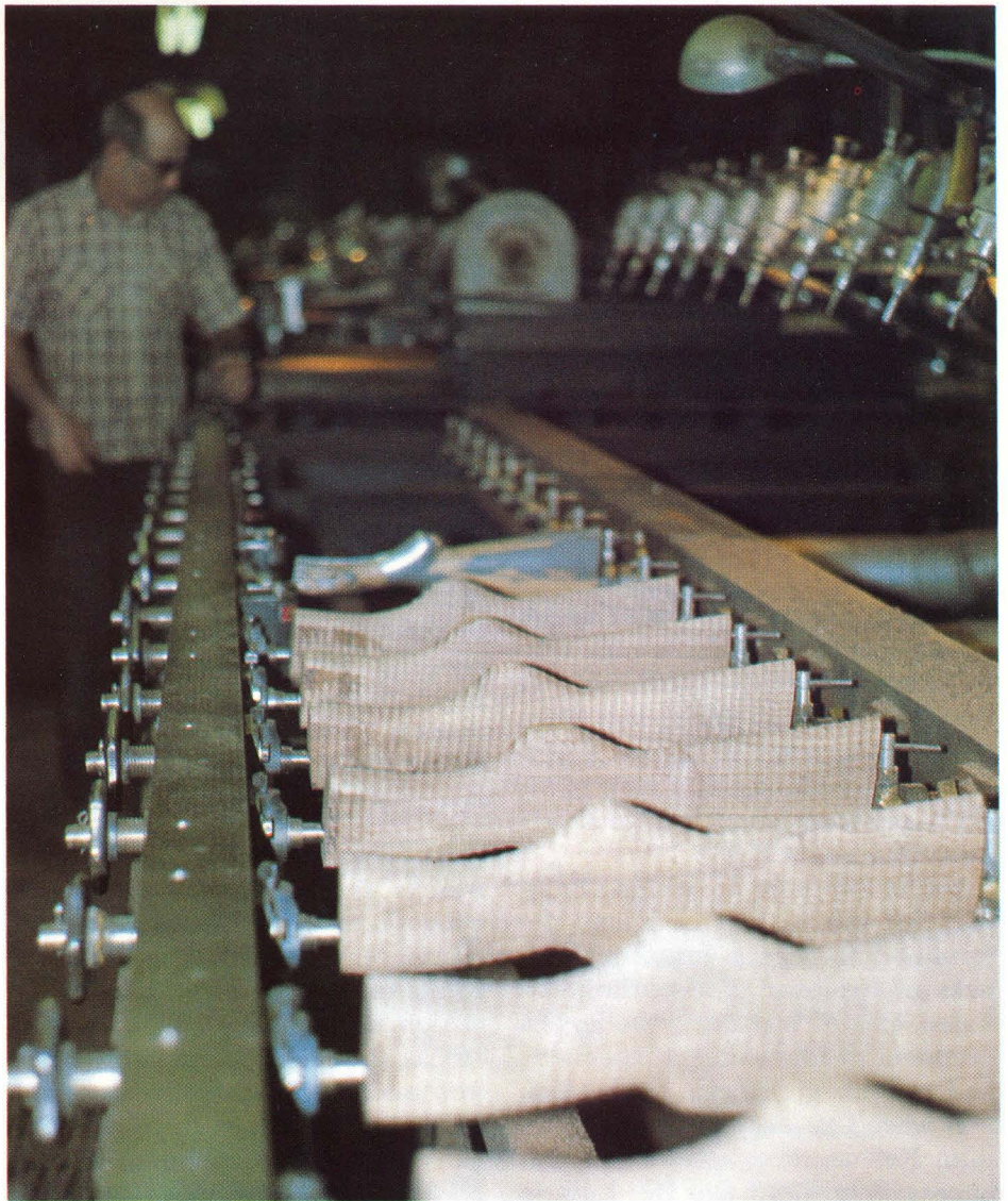
Once a walnut log is cut into slabs, the gunstock begins to take shape. A template is used to trace gunstock outlines on slabs (left). Band sawyers then convert the slabs to gunstock blanks, which are rough shaped by fixed routers as the blanks slowly rotate in carving machines (right). After butt plates and fittings are attached, stocks are smoothed with hand-held sanders (below right) and checkering is carved into the wood (below center). Gunstocks are sold according to grade (below left); common grade, fiddle-back figure, and the highly valuable feather figure illustrate the variable range, and expense, of gunstock options available to gun buyers. (Photo at left by John Strickler; all other photos by Mike Blair)
